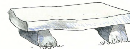
STONE BASE WITH CONCRETE TOP
